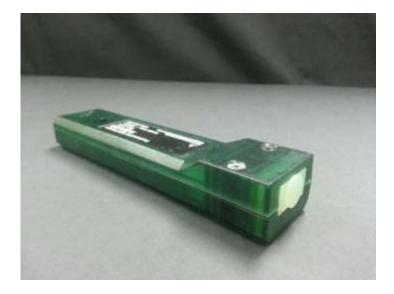
The sensor has a light-sensing element in the center, so the sensor should face the light source directly, and the experimental setup should ensure the sensor and light source are at the same height.
